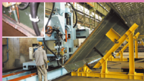
●I 桁溶接装置 I Beam Welding Equipment
